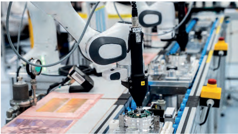
A snapshot from TQ's elegantly automated screw fastening solution.
