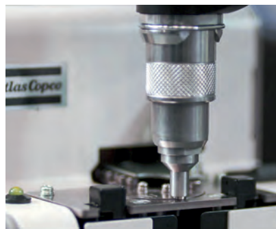
The end effector uses Panda's sensitivity to pick and fasten the screws successfully.
